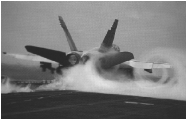
Fig 4: A F-18 Hornet in a carrier cat-shot aboard the USS Enterprise. Steam from the catapult form vortices at the wing tips. The main wing is producing positive lift, hence the counter clockwise vortex, the tail is producing negative lift thus it's tip vortex rotates in the opposite direction. Judging from the size of the vortices, not much positive net lift is available, but a lot of nose up moment is.
